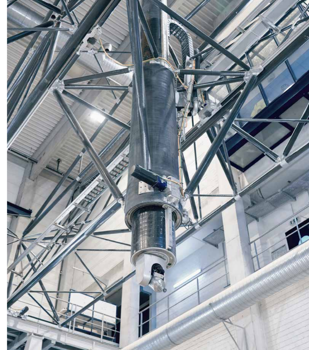
This completely revamped portal machines the lower workpiece heights of approximately 1 m to 4 m.
