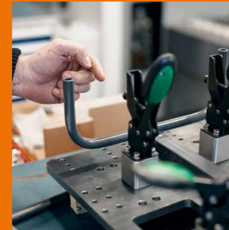
Test assembly of the welding template with shear clamps and inserted mounting unit.
